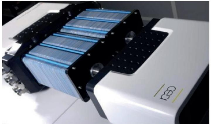
Fig. 1 A stack of a fuel cell. Credit: CEA
