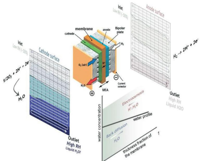
Fig. 2 Schematic representation of the 3D water repartition in a PEMFC single cell. Water is heterogeneously distributed in-plane (at the surface of the anode/cathode) and through-plane (across membrane thickness). Results were obtained from in-operando SANS measurements.
