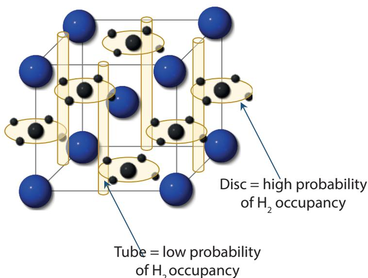
Fig. 2 A view of the atomic structure of the material under study. Neutron diffraction techniques pinpoint sites of hydrogen occupancy.
