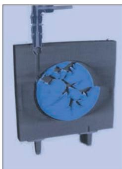
**A neutron tomography image.** It reveals the development of defects in a **light metal hydride storage material**: channels developing inside a hydrogen tank after two cycles of loading and unloading with hydrogen.
