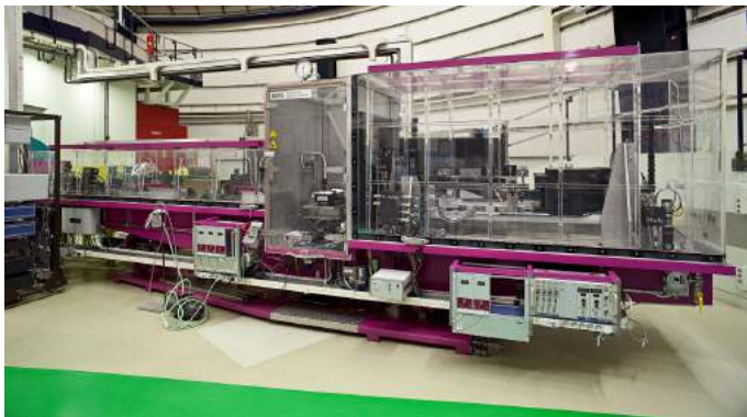
Figure 6: Cold source and new primary spectrometer will yield 1 to 2 orders of magnitude in flux. A 1D detector for off-specular will be needed in 2019.
