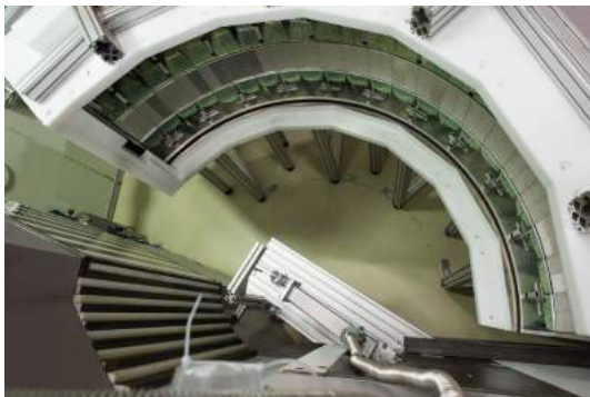
Figure 4: STFC/RAL design wavelength-shifting fiber {}^6\text{LiFZnS} detector consisting of 1408 pixels of 2.1mm wide, 200mm tall. Gamma/neutron discrimination better than 10^{-6} ( Sykora et al. IEEE Nucl.Sci.Symp. (2012) p.1567)
