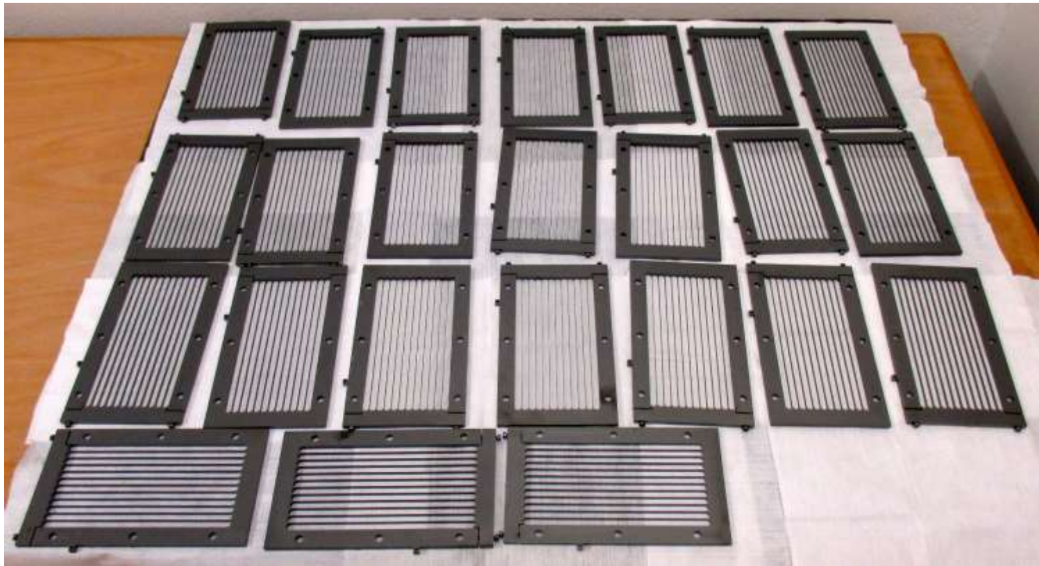
24 frames of thin walls for the mounting of a detector
