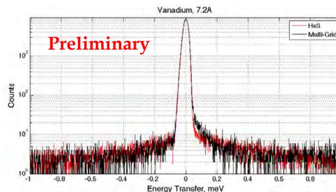
*Comparison between the He-3 and MultiGrid TOF peak recorded with the V sample at the CNSC.*
