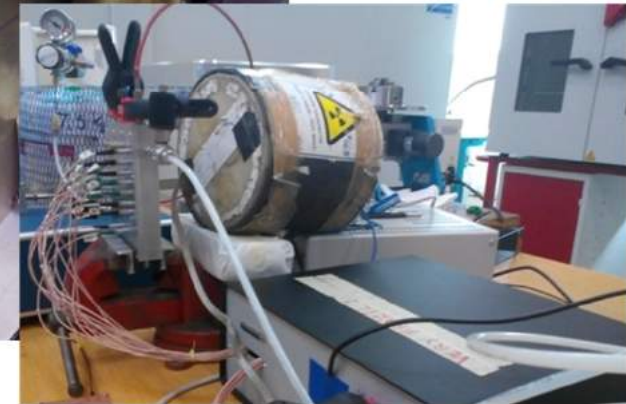
Debugging tests with a Am/Be neutron source, before moving the detection system into the Reactor Area.
