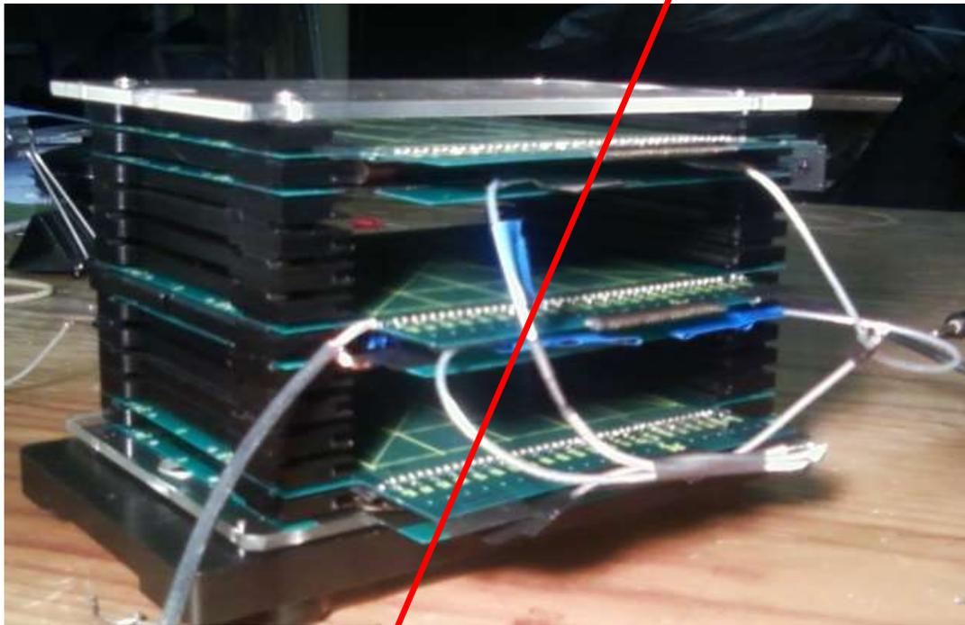
Simultaneous position resolution of  $38 \mu\text{m}$  and time resolution of  $80 \text{ ps}$  with cosmic rays
