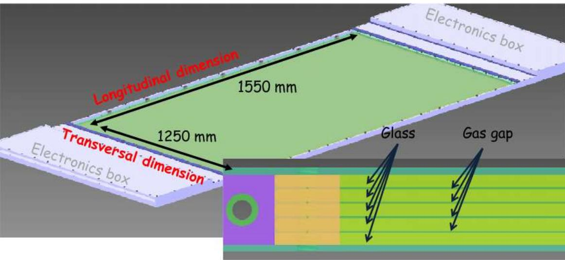
Large area (~2 m<sup>2</sup>) RPC detectors capable of measuring time and 2D position at the same time Readout by 53 channels/layer (time+charge)
