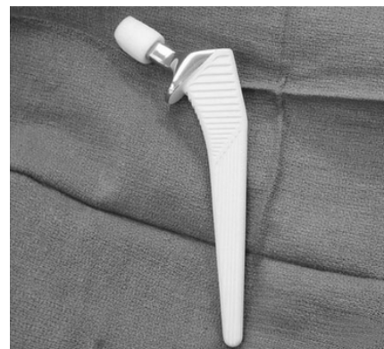
Figure 1. A femoral implant with hydroxyapatite coating. Picture from Cho et al, Clin. Orthop. Surg., 2010
