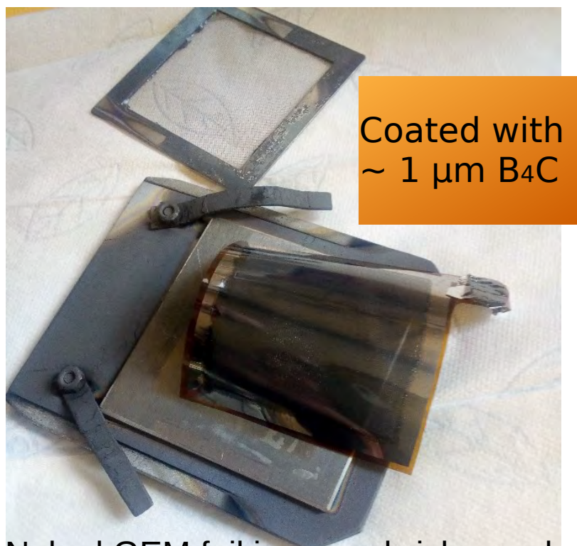
Naked GEM foil in a sandwich panel – mesh mask and protected plate –
