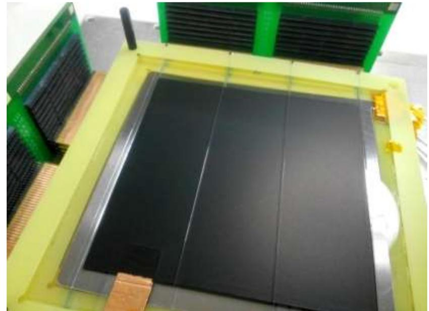
**Glass plate** (outer surface lined with a resistive layer) facing an **Al plate**
