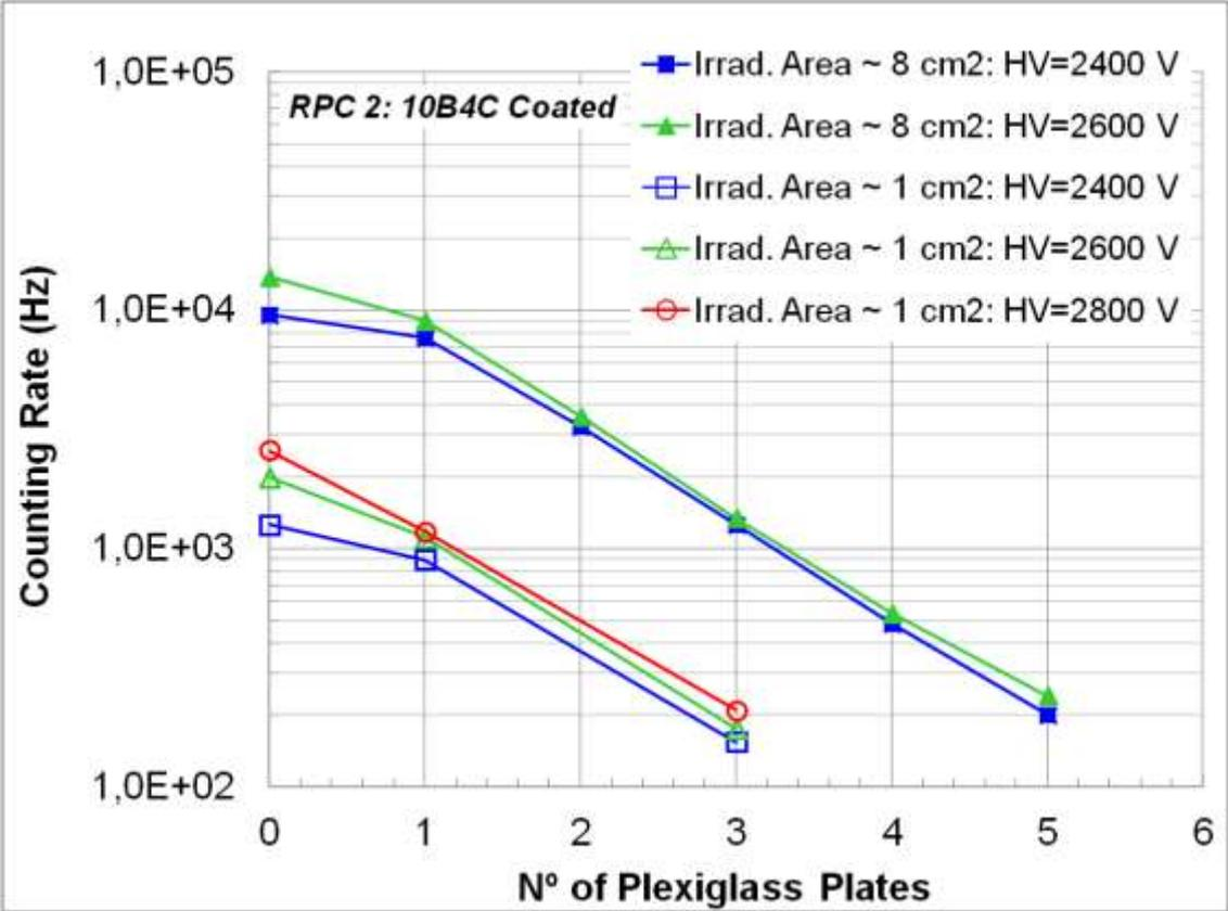
Attenuators: Plates of Plexiglass 3mm thick
