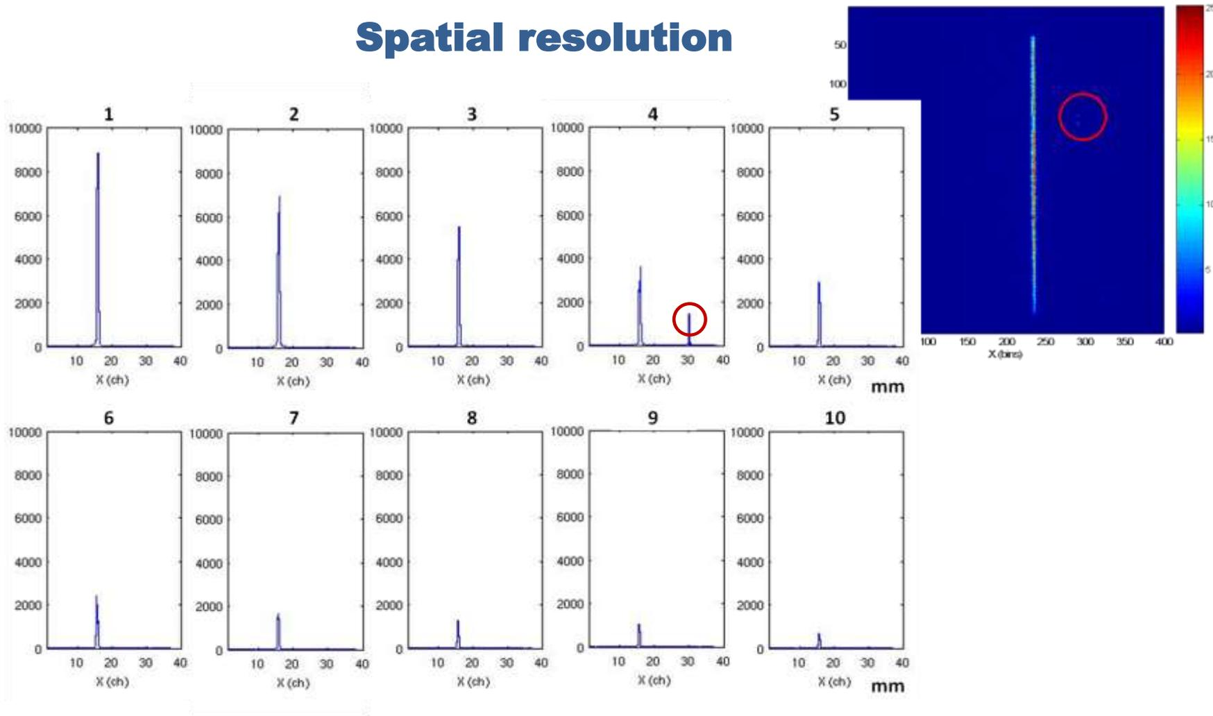
Data acquired with a vertical Cd slit (0.1 mm x 35 mm)
