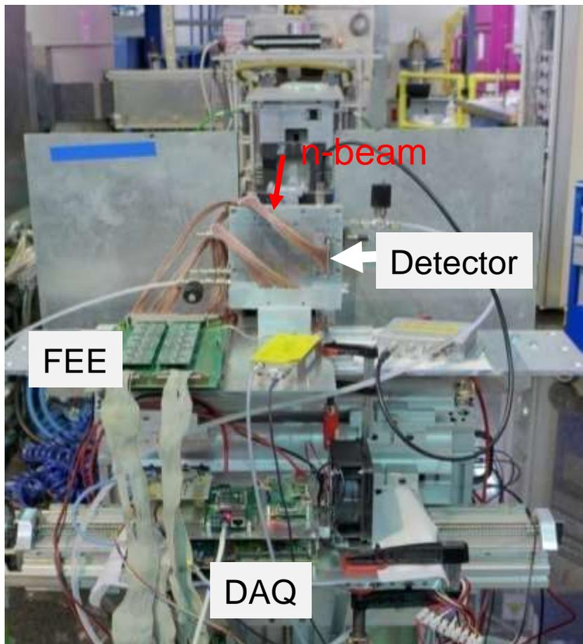
Detector prototype at TREFF neutron beam line ( $\lambda = 4.7 \text{ \AA}$ )
