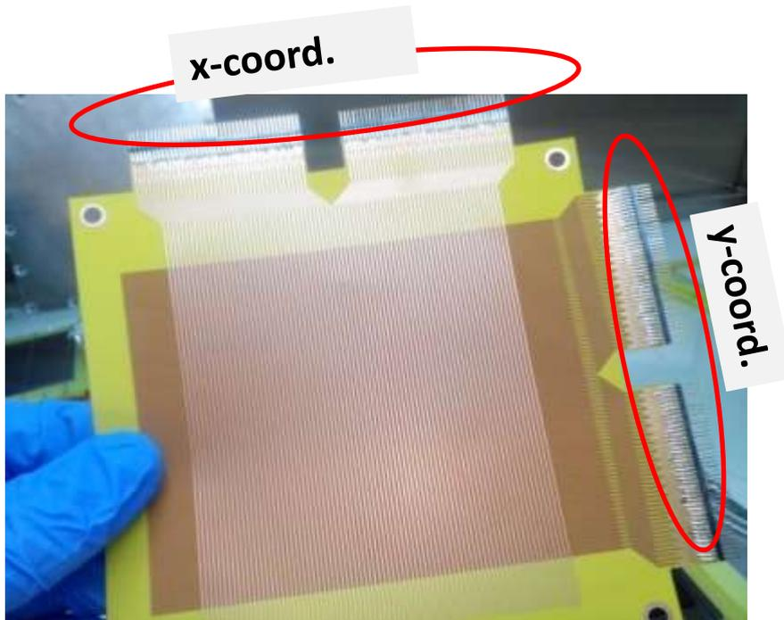
Thin Kapton PCBs with 3 layers of Cu-strips mutually orthogonal
