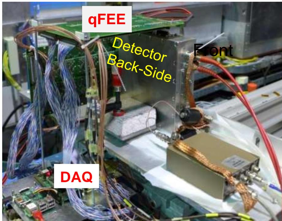
Prototype seated on the moving stage at TREFF ( $\lambda = 4.7 \text{ \AA}$ )
