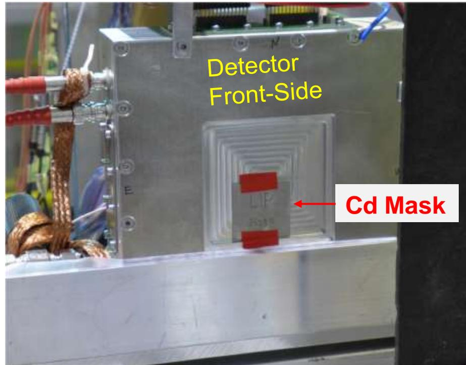
Aluminium gas-tight vessel (1mm thick neutron entrance window)
