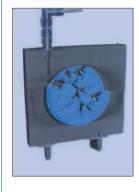
A neutron tomography image. It reveals the development of defects in a light metal hydride storage material: channels developing inside a hydrogen tank after two cycles of loading and unloading with hydrogen. Dehydrogenation pathways in an  $H_2$ **storage material**. Powder neutron diffraction experiments on a lithiumhydride / germanium composite (LiH / Ge) can reveals the species that form as the composite decomposes when slowly heated to 500°C.
