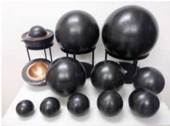
SINE2020-developed BSS-system with PE moderators, Cu and Pb shells
