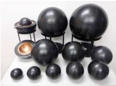
BSS-system with PE moderators and Cu shells
